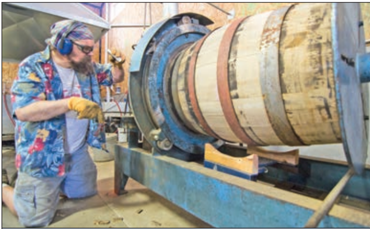
Rogue's cooper, Nate Lindquist, creates barrels on a machine called a crozer- one end holds the barrel in place, and the other has spinning blades that cut a perfect groove inside the barrel.
